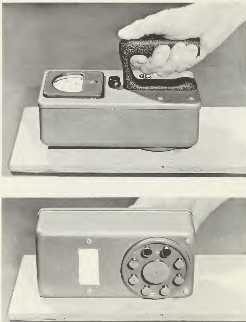
Figure 10. --A radio-frequency power-loss type of moisture meter.
